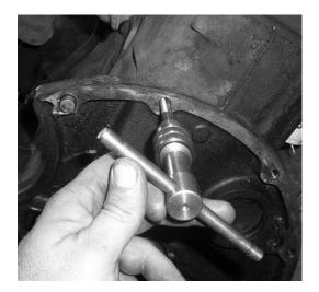
4. USING THE SUPPLIED 7/16-14 AND THE 3/18-16 BOLTS BOLT THE ADAPTER PLATE TO THE BLOCK. IF NECESSARY USE A RUBBER MALLET TO FIT THE PLATE UP TO THE BLOCK FLUSH. DO NOT USE THE CAP SCREWS TO FORCE THE PLATE ONTO THE BLOCK. CHECK FOR FIT. THE PLATE SHOULD FIT FLAT THE PLATE SHOULD FIT FLAT TO THE ENGINE BLOCK WITH NO ROCKING OR GAP.
