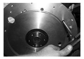
5. ONCE THE ADAPTER PLATE IS FLUSH, MARK THE PLATE FOR ANY TRIMMING OR CUTTING FOR CLEARANCE. IF THE PLATE WILL BE TRIMMED, BE CAREFUL NOT TO CUT TOO CLOSE TO ANY OF THE FASTENER HOLES AND REMOVE ANY BURRS LEFT FROM CUTTING.
