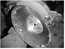
8. CAREFULLY ALIGN THE HUB SPACER/FLEX PLATE AND THE CRANKSHAFT BOLT HOLES WHILE PLACING THE HUB SPACER ONTO THE CRANKSHAFT. THE HUB SPACER SHOULD BE A CLOSE FIT TO THE CRANKSHAFT. INSTALL THE CRANKSHAFT BOLTS AND TORQUE TO THE PROPER VALUE.
